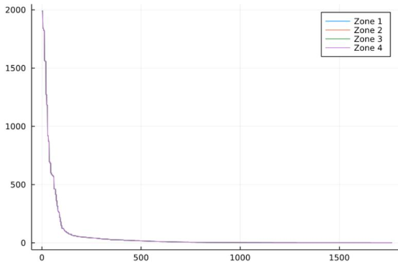
Figure 17 - Reserve price duration curve of the system using both approaches for the multi-area model with a separate ORDC in every zone. These results are provided only for simulation case 6 (10% of expensive hydro without strategic reserve being accounted for).
