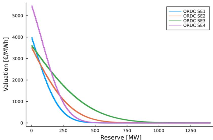
Figure 13 – ORDC function for each zone of Sweden for an assumed system  $\lambda$  of 0 €/MWh.
