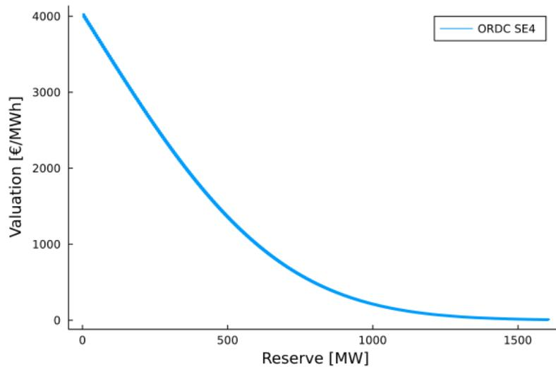
Figure 8 – ORDC function in SE4 based on Swedish system imbalances for an assumed system lambda of 0 €/MWh in a multi-area setup.
