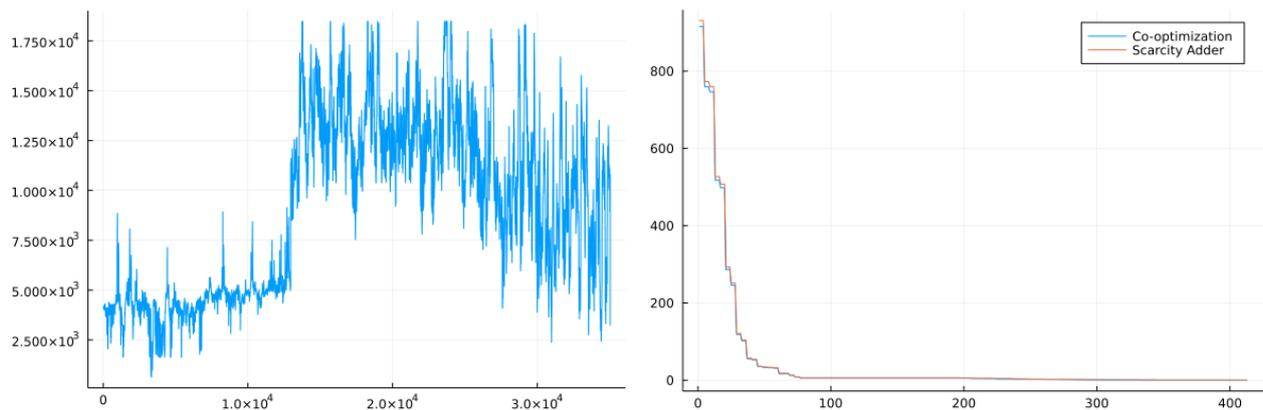
Figure 7 – On the left, the evolution of the total available reserve in the system in MW. On the right, the reserve price duration curve of the system using both approaches. These results are provided for the simulation case 6 (10% of expensive hydro without strategic reserve being accounted for).
