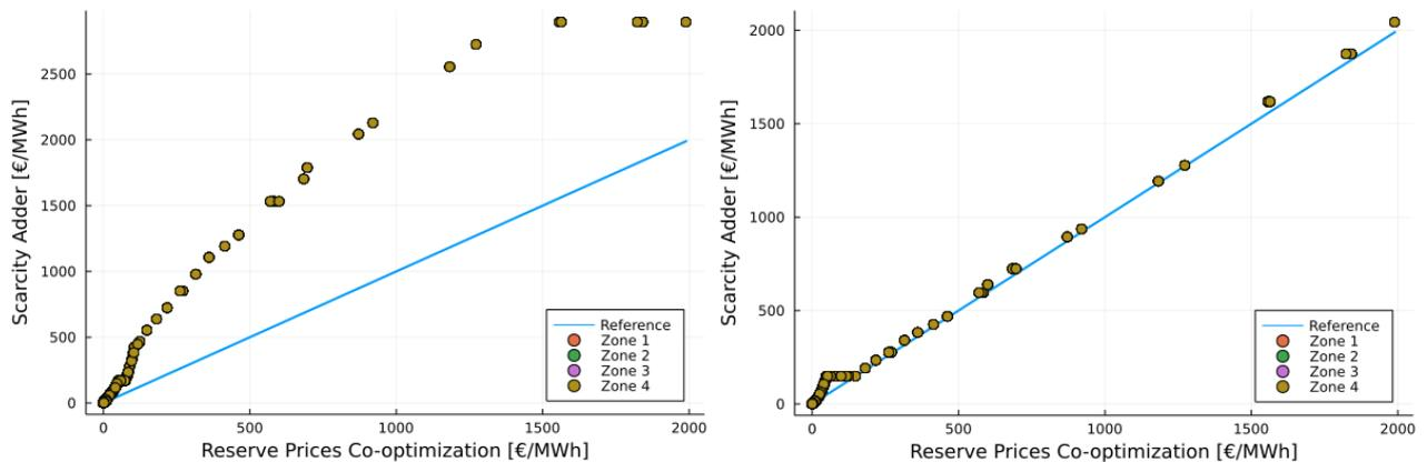
Figure 15 - Comparison of reserve prices obtained for the two approaches represented by the dots without (left) and with (right) 10% of expensive hydro power. The blue line corresponds to the reference on which the dots should land if the two approaches are providing identical results.
