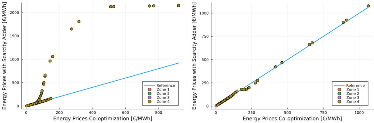
Figure 10 - Comparison of energy prices obtained for the two approaches represented by the dots without (left) and with (right) 10% of expensive hydro power. The blue line represents the reference on which the dots should land if the two approaches are providing identical results.
