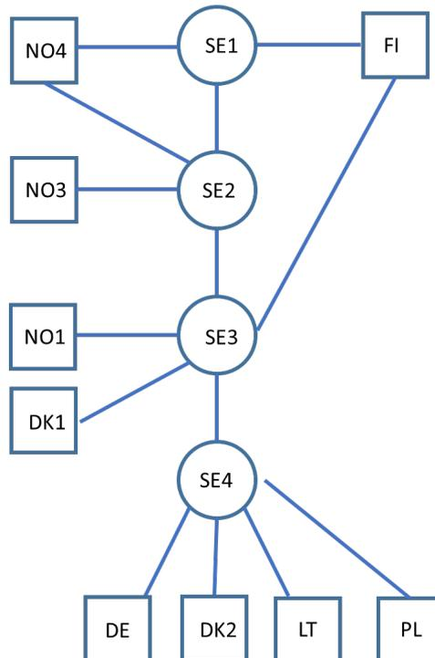
Figure 3 – Interconnections of Swedish system to zones out of Sweden. Circles indicate Swedish zones, boxes indicate zones out of Sweden.
