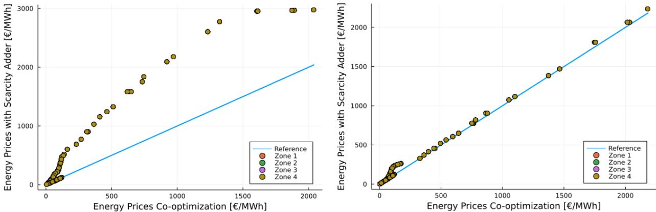
Figure 16 - Comparison of energy prices obtained for the two approaches represented by the dots without (left) and with (right) 10% of expensive hydro power. The blue line corresponds to the reference on which the dots should land if the two approaches are providing identical results.
