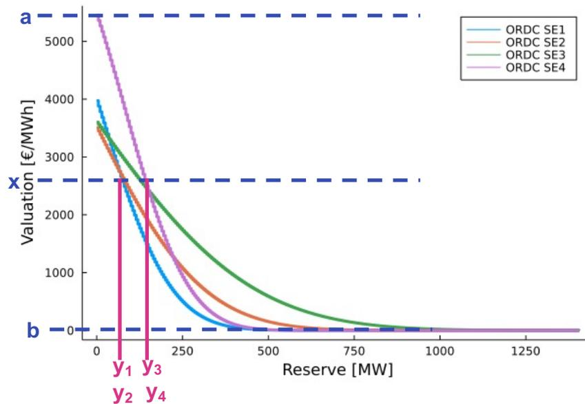
Figure 14 – Illustration of the different steps of the bisection algorithm used for computing the scarcity adder value for the multi-area case study with separate ORDCs in each zone.
