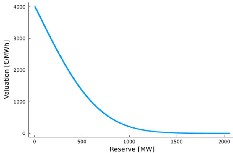
Figure 2 – ORDC based on Swedish system imbalances for an assumed system lambda of 0 €/MWh.
