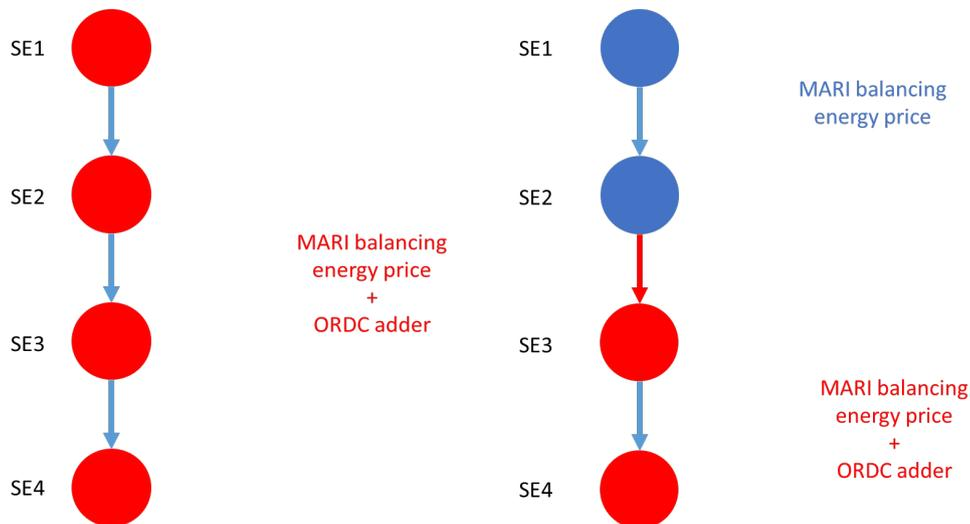
Figure 9 – Scarcity pricing in the multi-zone system of Sweden. Red circles represent nodes where a scarcity adder applies, whereas blue circles represent nodes where a scarcity adder does not apply. Blue arrows indicate links which do not experience congestion, whereas red arrows indicate links which do experience congestion.
