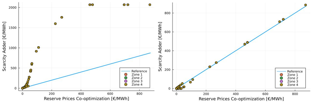
Figure 11 - Comparison of reserve prices obtained for the two approaches represented by the dots without (left) and with (right) 10% of expensive hydro power. The blue line represents the reference on which the dots should land if the two approaches were providing coherent results.
