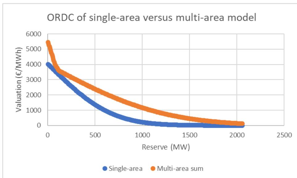
Figure 18 - Comparison of the ORDC curve used for the single-area model against the horizontal sum of the different ORDCs of the different zones in the multi-ORDC model.
