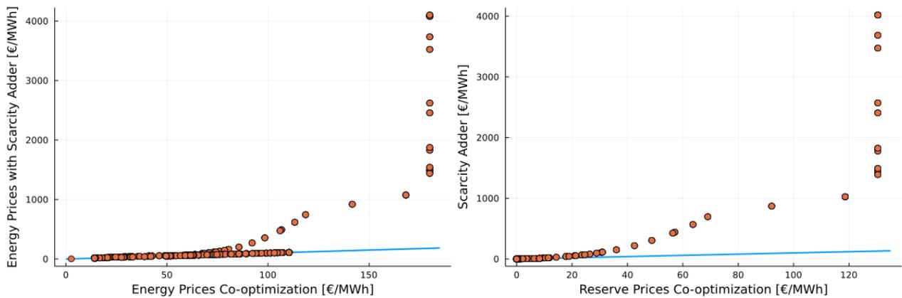
Figure 4 – Comparison of the energy (left) and reserve (right) prices obtained for the two approaches are represented by the dots. The blue line corresponds to the reference on which the dots should land if the two approaches are providing identical results.
