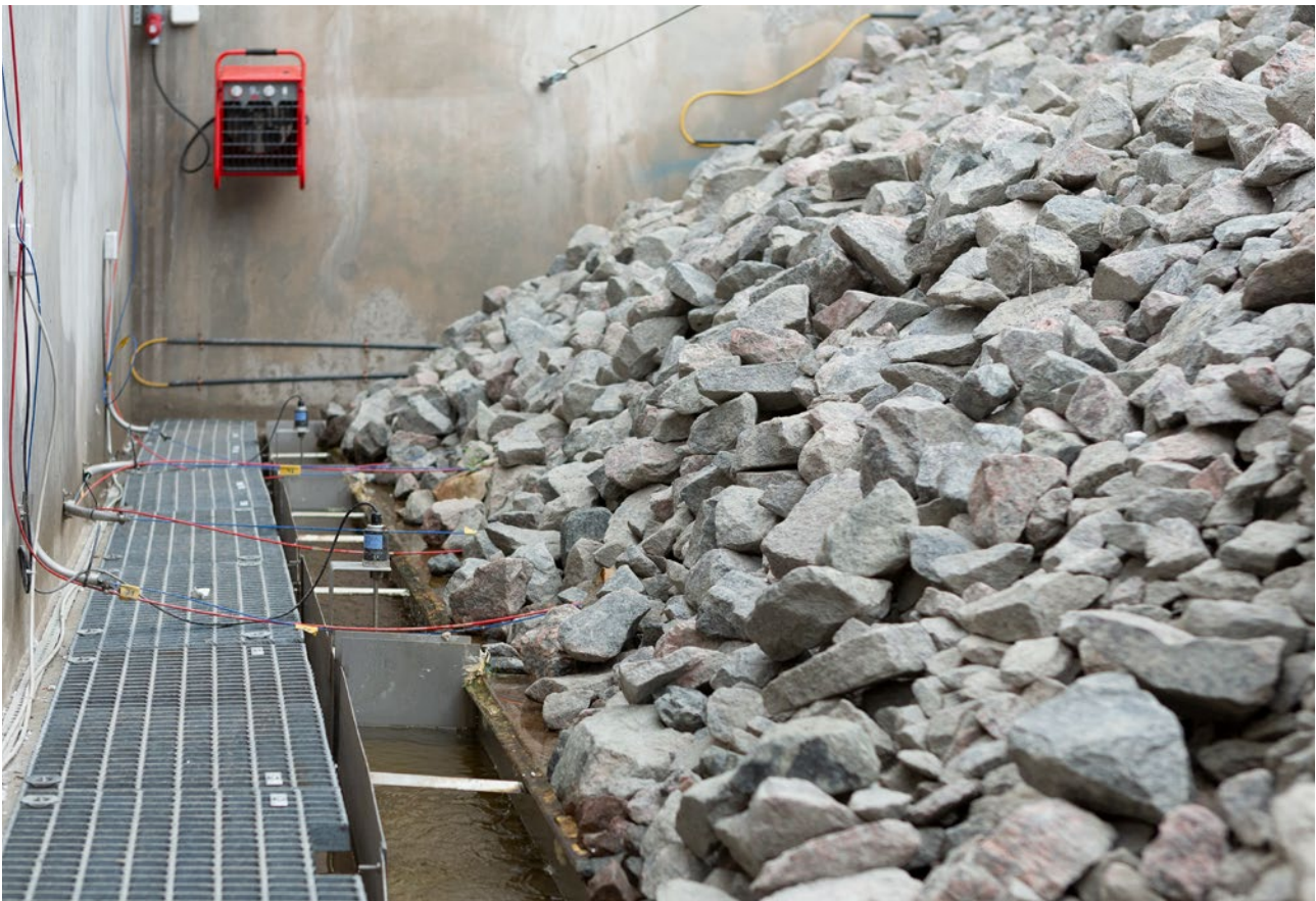
The experimental embankment dam at Vattenfall's laboratory facilities in Älvkarleby is utilized for research into damage detection methods. The dam was designed and constructed following the Swedish dam safety guidelines but has six built-in defects that could cause a dam failure. Photo: Svenska kraftnät.
