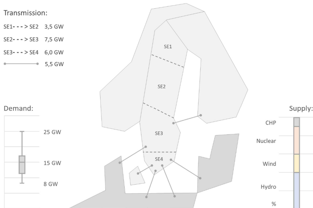
Figure G-1: Representation of the Nordic synchronous area and data for the Swedish power grid
