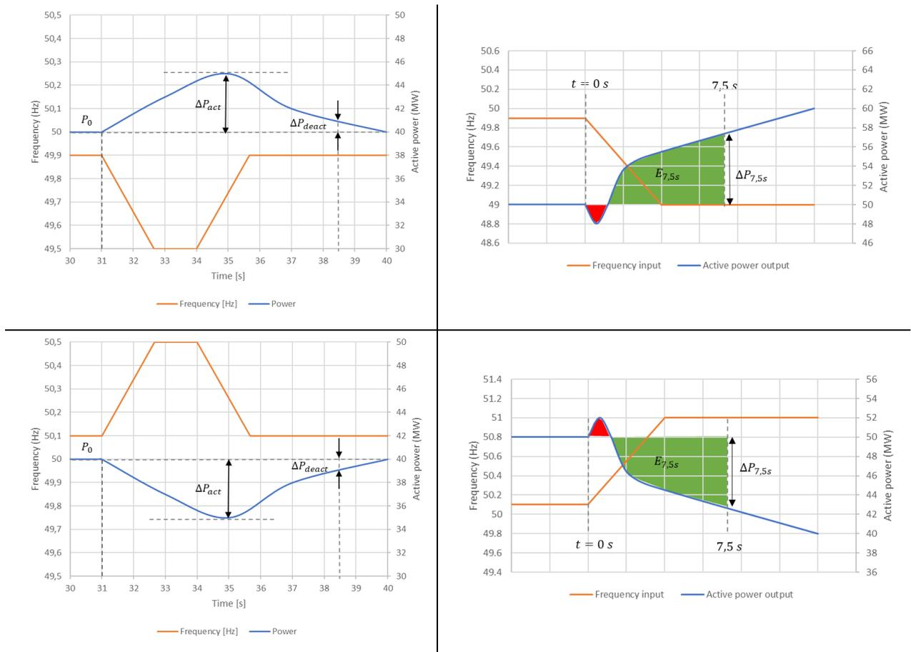
Figure 4. The left column shows the activation/deactivation requirements on ramp 1 and 2 for FCR-D upwards (top) and FCR-D downwards (bottom). The right column shows the dynamic performance requirements on ramp 5 for FCR-D upwards (top) and FCR-D downwards (bottom). The green area indicates positive energy contribution while the red area indicates negative energy contribution.
