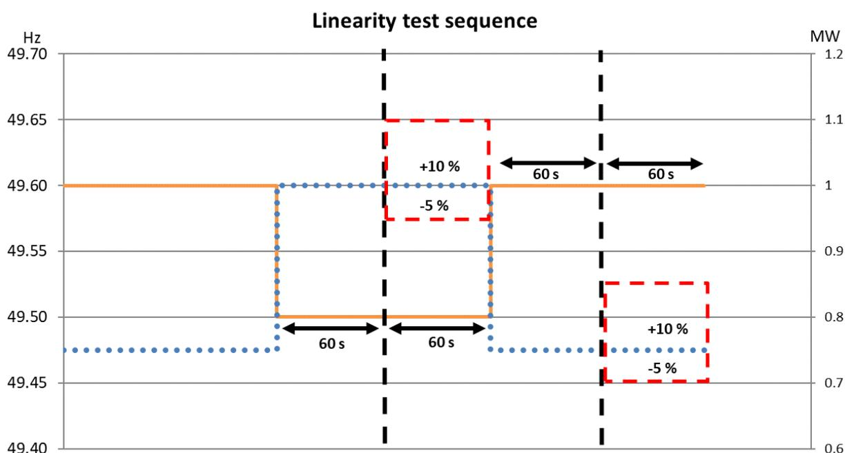
Figure 17. Allowed response area for FCR-D for the frequency steps from 49.6 Hz → 49.5 Hz → 49.6 Hz. The orange line is the frequency step. The blue dotted line is the directly proportional FCR response per MW. The red dashed squares indicate the allowed response area.
