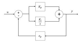
Figure 26. PI controller with droop.
