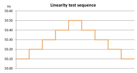
Figure 16: Grid frequency test signal for the FCR-D downwards linearity test.
