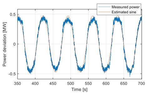
Figure 10. Example of the measured power from a sine test and the fitted sine.
