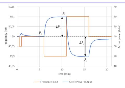
Figure 2. FCR-N step-response sequence. Input frequency (orange) and example response (blue).
