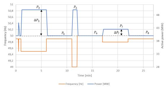
Figure 3. Illustration of FCR-D upwards ramp test. Here, FCR-N is inactive and therefore  $P_8 = P_6$ .
