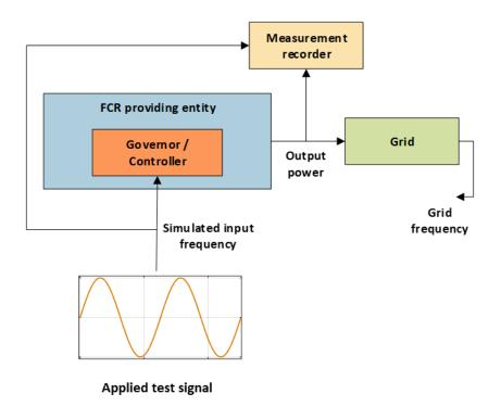
Figure 25. Test setup.
