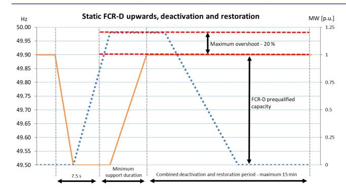
Figure 5. Maximum allowed overshoot and range for deactivation and restoration for static FCR-D. The orange line is an arbitrarily frequency ramp chosen to illustrate an allowed response from static FCR-D. The blue dotted line is an allowed response from static FCR-D.
