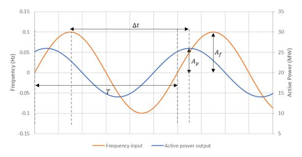
Figure 7. Example response (blue) from input frequency (orange) for FCR sine test.
