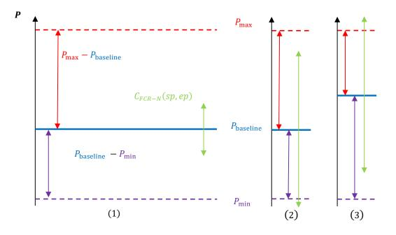
Figure 19. The three limits of FCR-N capacity for an entity which is limited either by prequalification test result (1), minimum active power (2) or maximum active power (3).
