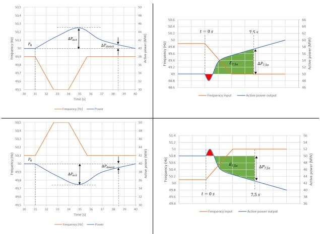
Figure 4. The left column shows the activation/deactivation requirements on ramp 1 and 2 for FCR-D upwards (top) and FCR-D downwards (bottom). The right column shows the dynamic performance requirements on ramp 5 for FCR-D upwards (top) and FCR-D downwards (bottom). The green area indicates positive energy contribution while the red area indicates negative energy contribution.
