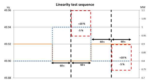
Figure 13. Allowed response area for FCR-N for the frequency steps from 49.92 Hz → 49.90 Hz → 49.92 Hz. The orange line is the frequency step. The blue dotted line is the directly proportional FCR response. The red dashed squares indicate the allowed response area.
