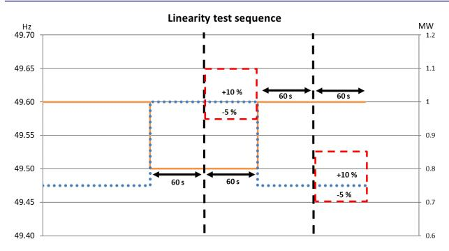
Figure 17. Allowed response area for FCR-D for the frequency steps from 49.6 Hz  $\rightarrow$  49.5 Hz  $\rightarrow$  49.6 Hz. The orange line is the frequency step. The blue dotted line is the directly proportional FCR response per MW. The red dashed squares indicate the allowed response area.
