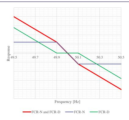
Figure 18. Steady state active power activation as a function of frequency, droop profile of FCR-N (blue), FCR-D (green) and both combined (red).
