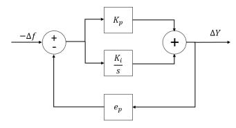
Figure 27. PI controller with droop where the Kp and Ki parameters are independent.
