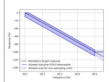
Figure 14. Activation of piecewise linear FCR-D resources. The black line indicates the mandatory target response. The controller shall be designed to minimise the deviation from the target response. The blue area defines the allowed outcome of the deviations, due to e.g. non-linear effects or step sizes for relay connected loads. The coordinates of the corners are provided in Table 8 below
