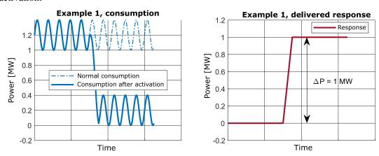
Figure 21. Example response where variations are independent of the delivered response.
