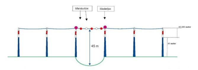
If the top line is higher than 45 metres above ground level or water level and crosses a large watercourse, valley, national or European route, the line must be marked with a warning ball with a diameter of 60 centimetres. This means that it is the greatest height of the line above ground level or water level that determines whether or not aviation marking on the line is necessary, not the height of the pylon.
