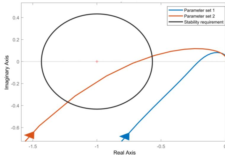
FIGURE 62: NYQUIST DIAGRAM FOR PARAMETER SET 1 AND 2 FOR A 120 GWs SYSTEM
