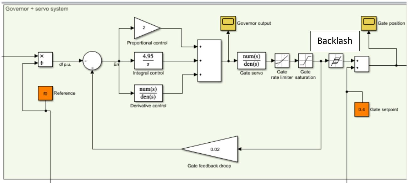
FIGURE 6. BLOCK DIAGRAM OF THE GOVERNOR AND SERVO.
