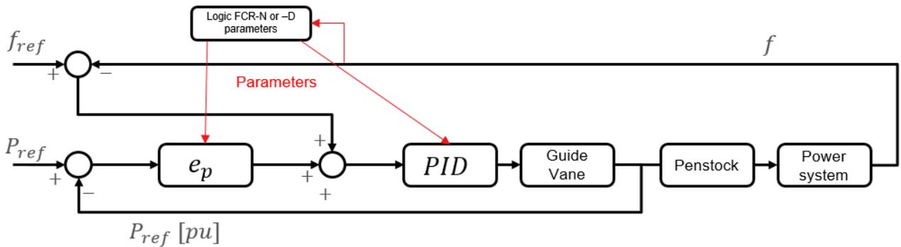
**FIGURE 31 SCHEMATIC (SIMPLIFIED) FREQUENCY CONTROL SYSTEM WITH GATE FEEDBACK AND SWITCHING OF PARAMETERS AT THE FREQUENCY THRESHOLD.**
