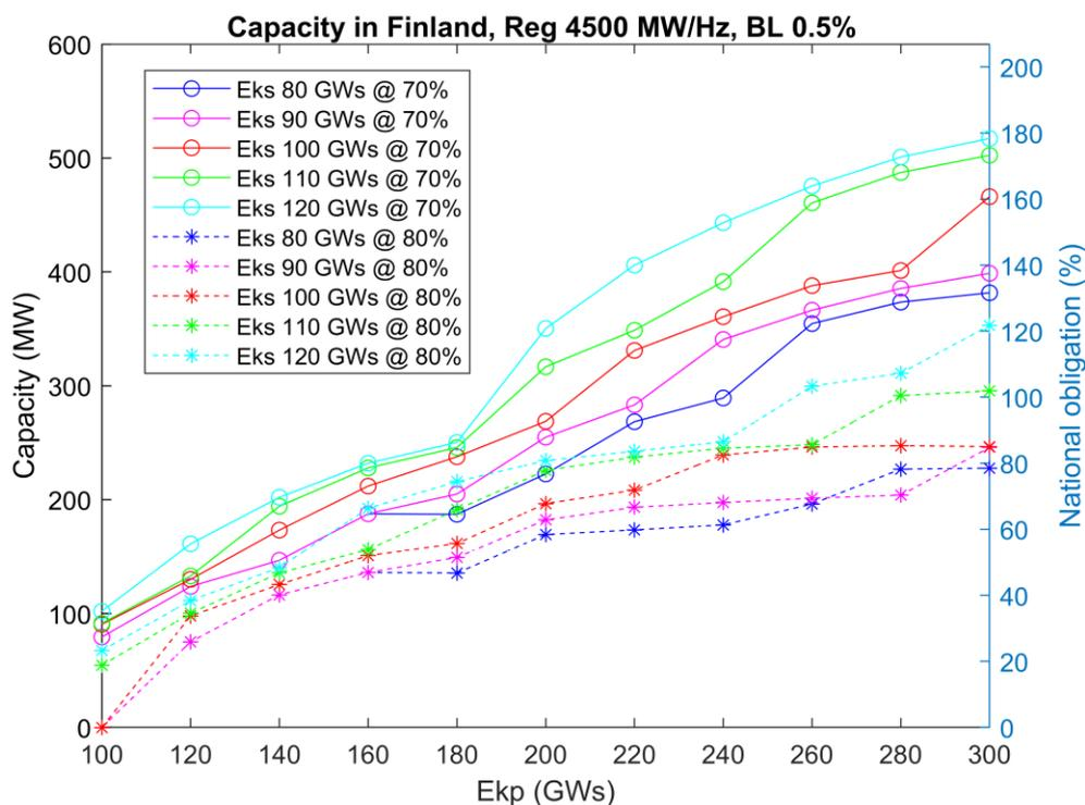
**FIGURE 11. ESTIMATED CAPACITY IN FINLAND BASED ON INSTALLED CAPACITY AND DISTRIBUTION OF WATER TIME CONSTANTS. LEFT Y-AXIS IS IN MW AND TO THE RIGHT IN PERCENTAGE OF NATIONAL OBLIGATION (290 MW [FCR MARKET LIQUIDITY NEEDS]). BACKLASH IS SET TO 0.5 % OF RATED MACHINE POWER.**
