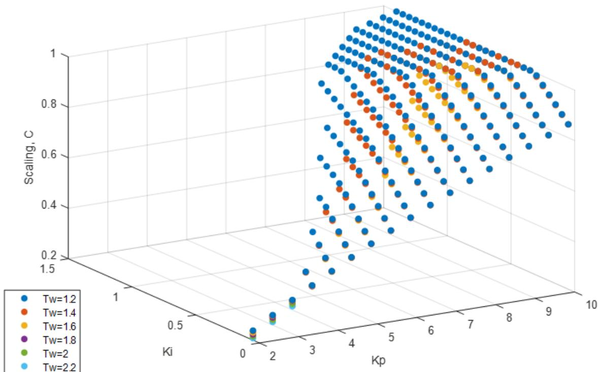
**FIGURE 4: 3D-PLOT OF CAPACITY PLOTTED AS A FUNCTION OF PROPORTIONAL GAIN,  $K_p$ , AND INTEGRAL GAIN,  $K_i$ , FOR DIFFERENT WATER TIME CONSTANTS,  $T_w$  (SEE LEGEND). EKS=90 GWS, EKP=300 GWS, BACKLASH=0.5% AND DROOP AT 4%.**
