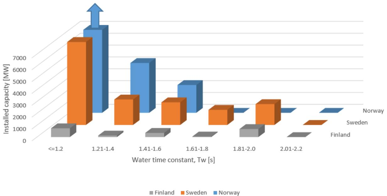
FIGURE 3: INSTALLED HYDRO CAPACITY IN THE NORDIC POWER SYSTEM DISTRIBUTED BY COUNTRY AND WATER TIME CONSTANT
