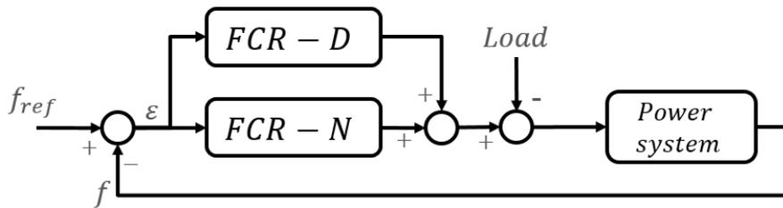
FIGURE 29 MODEL OF A SYSTEM WITH FCR-N AND -D SUPPLIED SEPARATELY.
