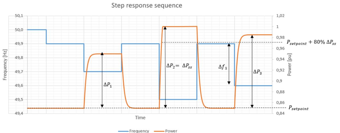
FIGURE 22: EXAMPLE OF PREQUALIFICATION TEST TO DETERMINE THE SATURATION FACTOR
