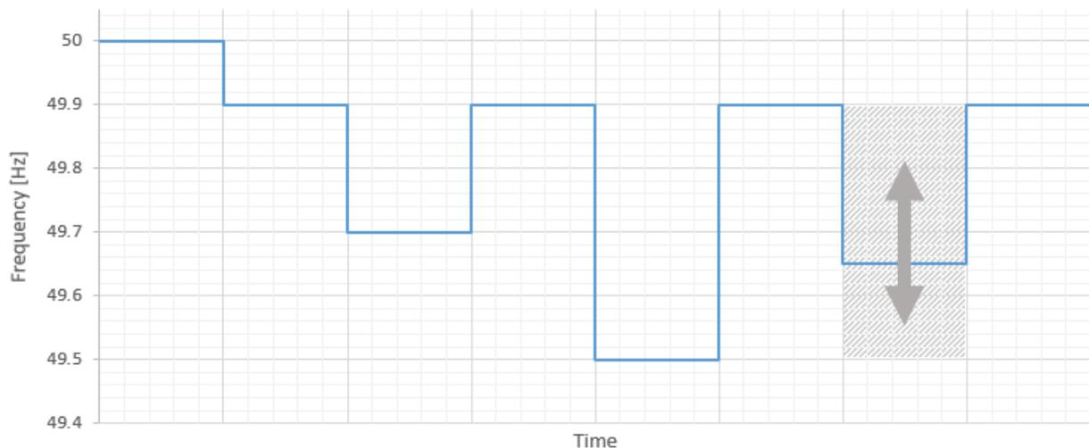
FIGURE 23: FCR-D UPWARDS REGULATION STEP RESPONSE SEQUENCE FOR UNITS SATURATING.
