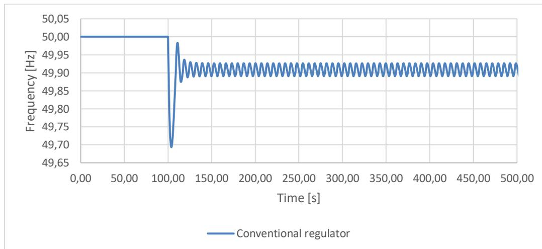
**FIGURE 37** FREQUENCY RESPONSE OF A SYSTEM WITH A CONVENTIONAL REGULATOR SWITCHING BETWEEN  $e_{p,FCR-N} = 0.08$  AND  $e_{p,FCR-D} = 0.04$ . THE IMPOSED POWER IMBALANCE IS 600 MW.
