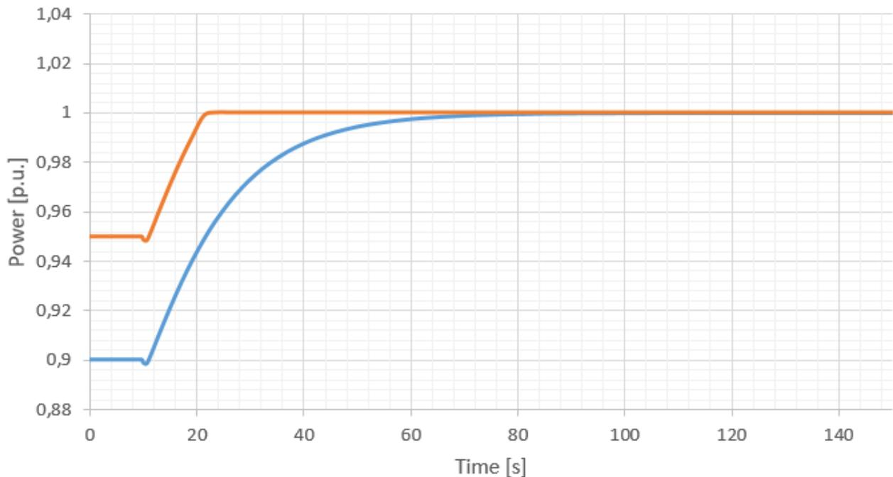
**FIGURE 18: EXAMPLE OF A -0.4 Hz STEP RESPONSE FOR A UNIT RUNNING THE TEST FOR DOCUMENTING THE STEADY STATE DELIVERY OF FCR-D, BUT WITH SATURATION DUE TO MAXIMUM POWER BEING REACHED.**
