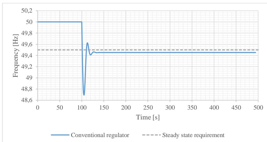
**FIGURE 35** FREQUENCY RESPONSE OF A SYSTEM WITH A CONVENTIONAL REGULATOR SWITCHING BETWEEN  $e_{p,FCR-N} = 0.04$  AND  $e_{p,FCR-D} = 0.08$ . THE IMPOSED POWER IMBALANCE IS 2050 MW.
