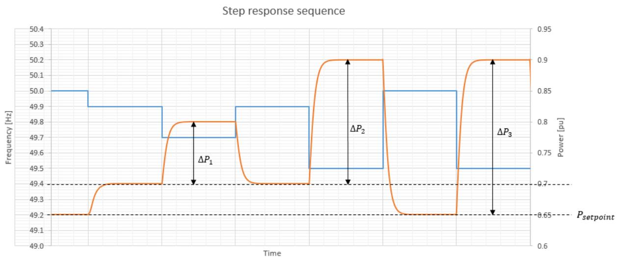
**FIGURE 55 EXAMPLE OF STEP RESPONSE FOR FCR-D UPWARDS REGULATION FOR DELIVERING BOTH FCR-N AND FCR-D**
