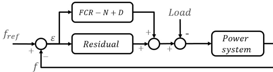
**FIGURE 30 MODELLING A SYSTEM WITH FCR-N AND -D PARTLY SUPPLIED FROM UNITS DELIVERING BOTH FCR-N AND -D, AND THE RESIDUAL FCR DELIVERED FROM A PARALLEL BRANCH.**
