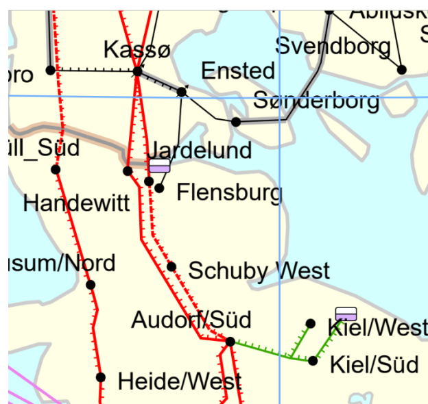
Figure 1: Topological overview of the Denmark West (DK1) – Germany (DE/LU) AC connection within CCR Hansa. Each red line represents a 380/400kV interconnector, consisting of a double circuit across the onshore border between Denmark (DK1)
