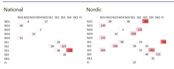
Figure 12. Total cost of allocated CZC for exchange of aFRR capacity (from = left row, to = upper header), 1000 EUR
