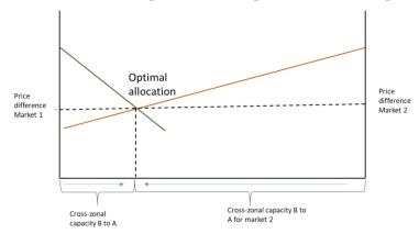
Figure 7. Bathtub diagram showing the optimal allocation of CZC between two markets
