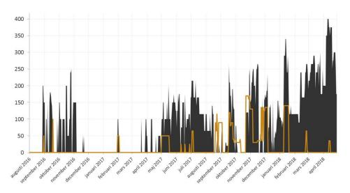
Figure 17: Cross-zonal capacity allocated for exchange of balancing services during the period from August 2016 to April 2018. The black line show cross-zonal capacity between SE2 and SE3. Yellow line shows cross-zonal capacity between SE3 and SE4. Source: Svenska kraftnät
