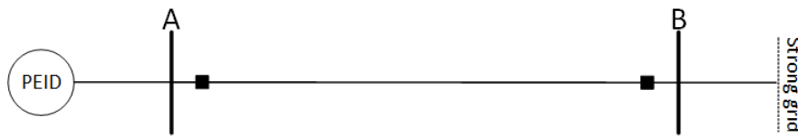
Figure 9.1: An example of a transmission line that integrates a PEID to a strong grid radially.
