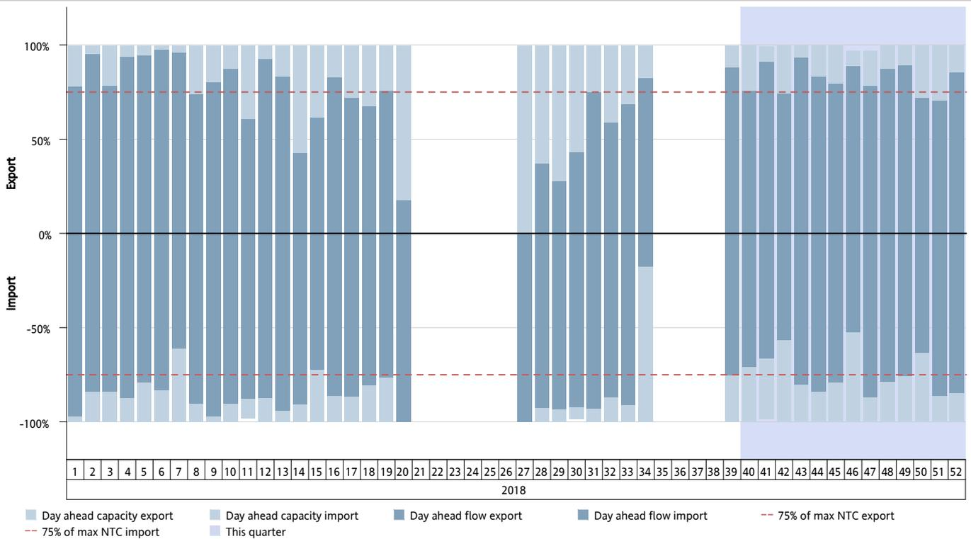
Figure 20: Shows cross-zonal day-ahead capacity result for the HVDC corridor DK2-DE, showing average weekly capacity given and flow as a percentage of max NTC. Available capacity is given for all hours, but the average flow is only given for hours with flow in that direction. Export indicates flow from DK2 to DE, while import indicates flow from DE to DK2.
