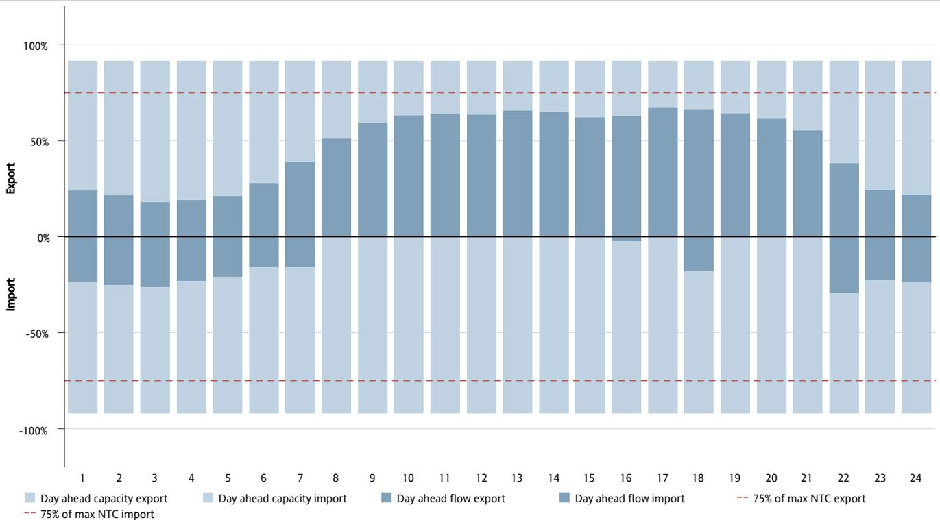
Figure 29: Shows cross-zonal day-ahead capacity result for the HVDC corridor FI-EE, showing average per hour of the day (1-24) capacity given and flow as a percentage of max NTC. Available capacity is given for all hours, but the average flow is only given for hours with flow in that direction. Export indicates flow from FI to EE, while import indicates flow from EE to FI.
