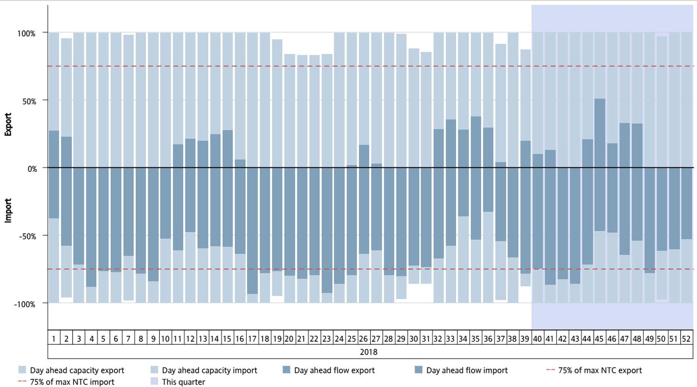
Figure 36: Shows cross-zonal day-ahead capacity result for the HVDC corridor FI-SE3, showing average weekly capacity given and flow as a percentage of max NTC. Available capacity is given for all hours, but the average flow is only given for hours with flow in that direction. Export indicates flow from FI to SE3, while import indicates flow from SE3 to FI.
