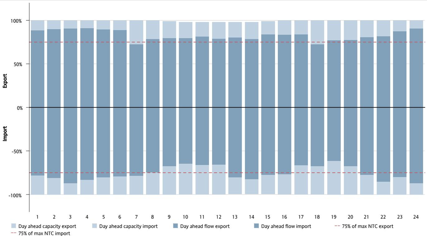
Figure 21: Shows cross-zonal day-ahead capacity result for the HVDC corridor DK2-DE, showing average per hour of the day (1-24) capacity given and flow as a percentage of max NTC. Available capacity is given for all hours, but the average flow is only given for hours with flow in that direction. Export indicates flow from DK2 to DE, while import indicates flow from DE to DK2.
