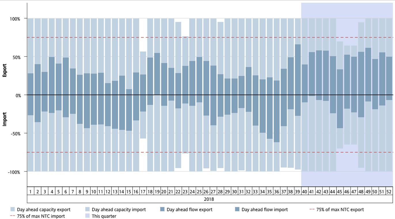
Figure 28: Shows cross-zonal day-ahead capacity result for the HVDC corridor FI-EE, showing average weekly capacity given and flow as a percentage of max NTC. Available capacity is given for all hours, but the average flow is only given for hours with flow in that direction. Export indicates flow from FI to EE, while import indicates flow from EE to FI.
