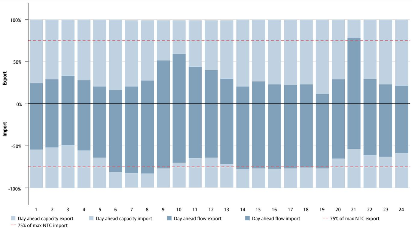
Figure 37: Shows cross-zonal day-ahead capacity result for the HVDC corridor FI-SE3, showing average per hour of the day (1-24) capacity given and flow as a percentage of max NTC. Available capacity is given for all hours, but the average flow is only given for hours with flow in that direction. Export indicates flow from FI to SE3, while import indicates flow from SE3 to FI.
