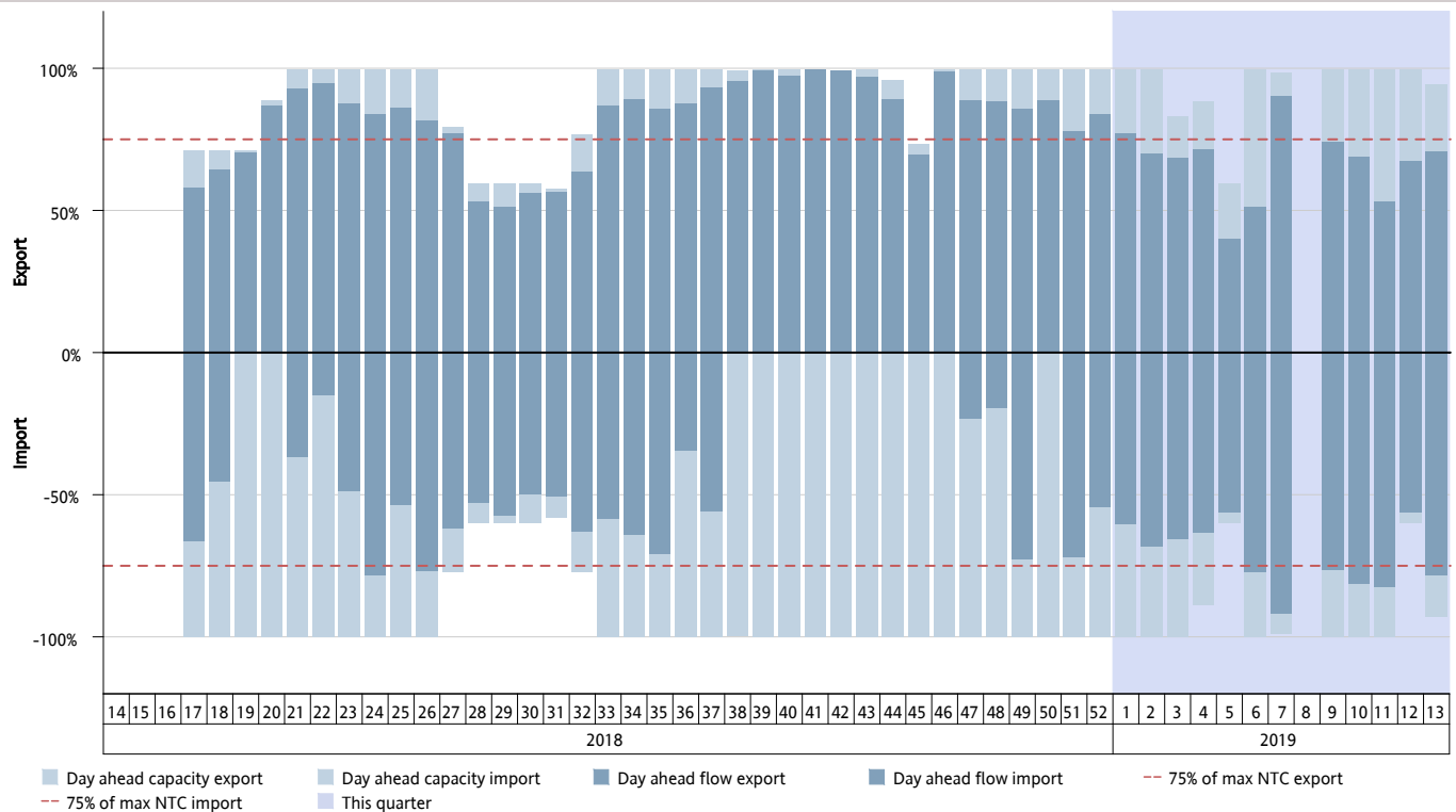
Figure 44: Shows cross-zonal day-ahead capacity result for the HVDC corridor NO2-NL, showing average weekly capacity given and flow as a percentage of max NTC. Available capacity is given for all hours, but the average flow is only given for hours with flow in that direction. Export indicates flow from NO2 to NL, while import indicates flow from NL to NO2.
