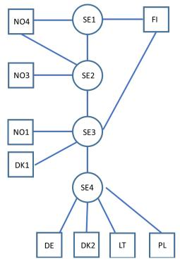
Figure 3 – Interconnections of Swedish system to zones out of Sweden. Circles indicate Swedish zones, boxes indicate zones out of Sweden.
