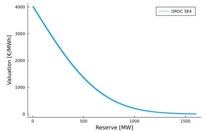
Figure 8 – ORDC function in SE4 based on Swedish system imbalances for an assumed system lambda of 0 €/MWh in a multi-area setup.
