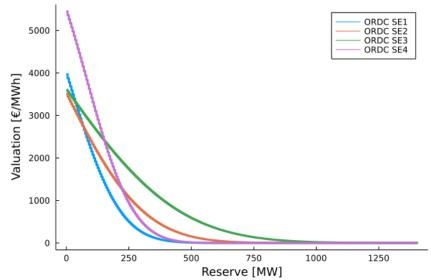
Figure 13 – ORDC function for each zone of Sweden for an assumed system lambda of 0 €/MWh.
