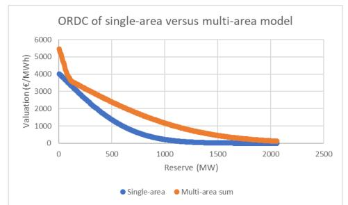
Figure 18 - Comparison of the ORDC curve used for the single-area model against the horizontal sum of the different ORDCs of the different zones in the multi-ORDC model.
